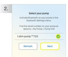
Make sure the pump is within close proximity to the phone. Once a connection is established, select the radio button next to the pump's serial number and tap Next.
