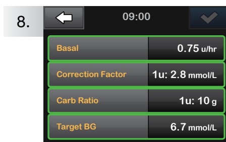
8. Tap Basal , Correction Factor , Carb Ratio , or Target BG to make changes, then tap Done . When you are finished, tap Save .
